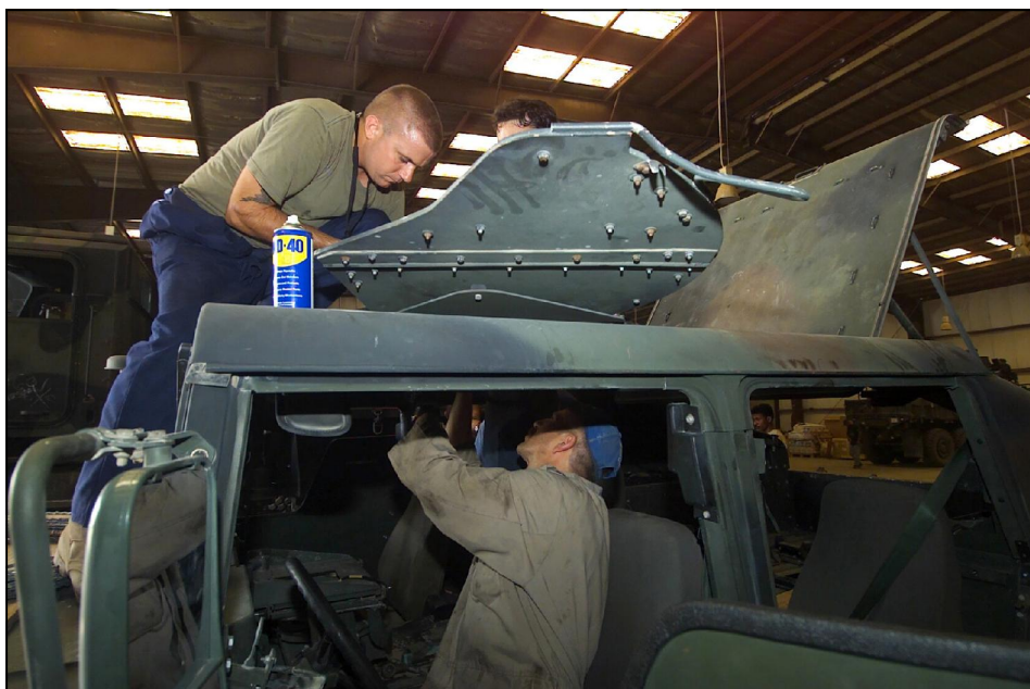
Civilian contractors install a gunner's shield atop a Humvee from the 24th Marine Expeditionary Unit at an armor installation facility in Kuwait on July 17, 2004.
